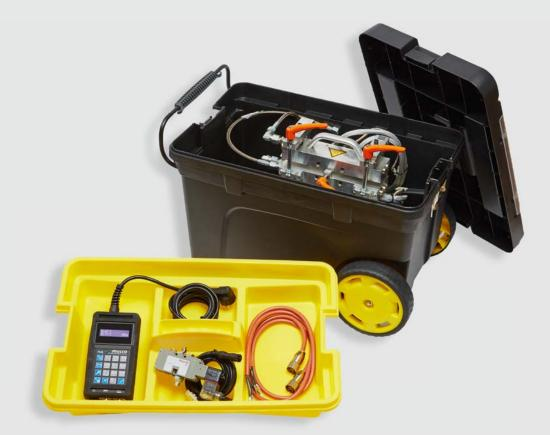
Even top-quality products will eventually wear out. The same applies to polyurethane timing belts which, from time to time, need to be replaced. We designed the portable TSG 5 welder to assist you in replacing drive units that take a lot of mounting effort and are difficult to access due to upstream machine components.
